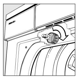
■ Use a 19 mm spanner to unscrew the plastic cover inside the drum above the door
